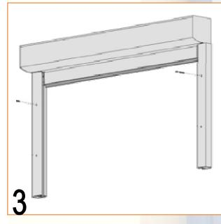
Put one screw into top install hole in guiderail on each side of frame, but leave screw slightly loose to hold into place until you can level out frame
